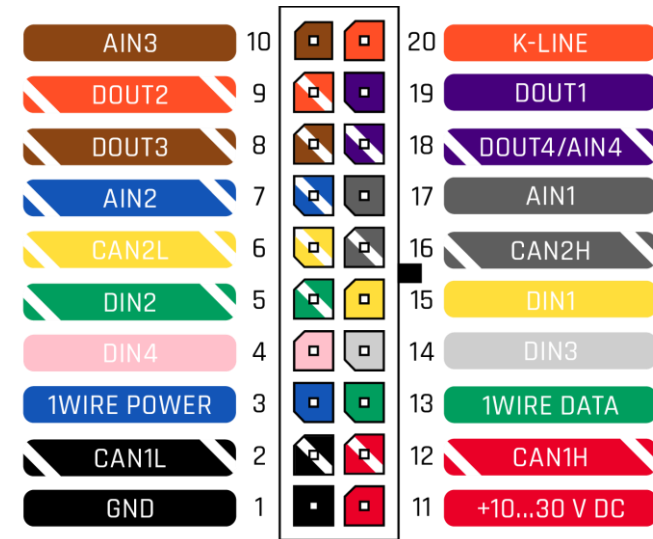
Figure 2 FMM640 pinout
